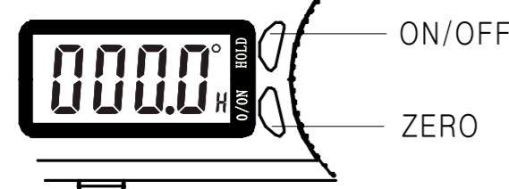
**ON/OFF** Short press ON/OFF to turn on the device. Short press ON/OFF to shut off the LCD. Long press ON/OFF for more than 3 seconds to shut off the whole system. Automatically shut off function in 6 min. Move the scale to turn on the device when at off LCD status.
